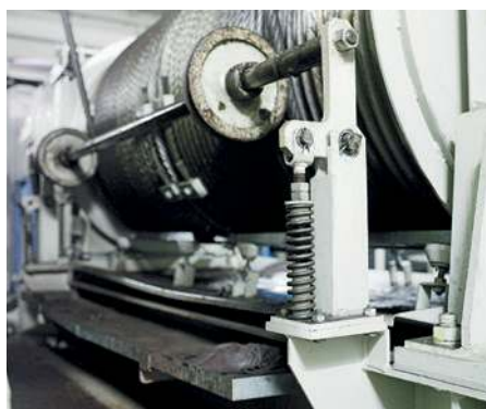
↑ Rope pressure device for safe winding of hoisting ropes
