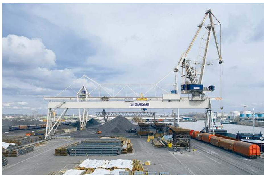
↑ Tukan with an asymmetrical gantry
