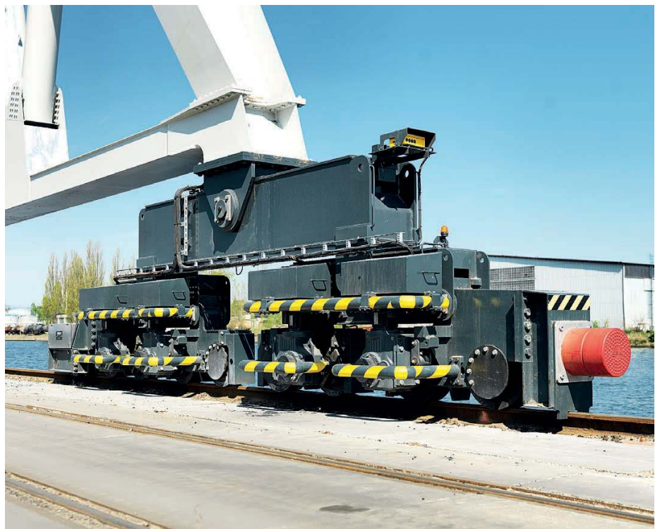
↑ Fully electric rail-borne travelling gears: safe and effective
