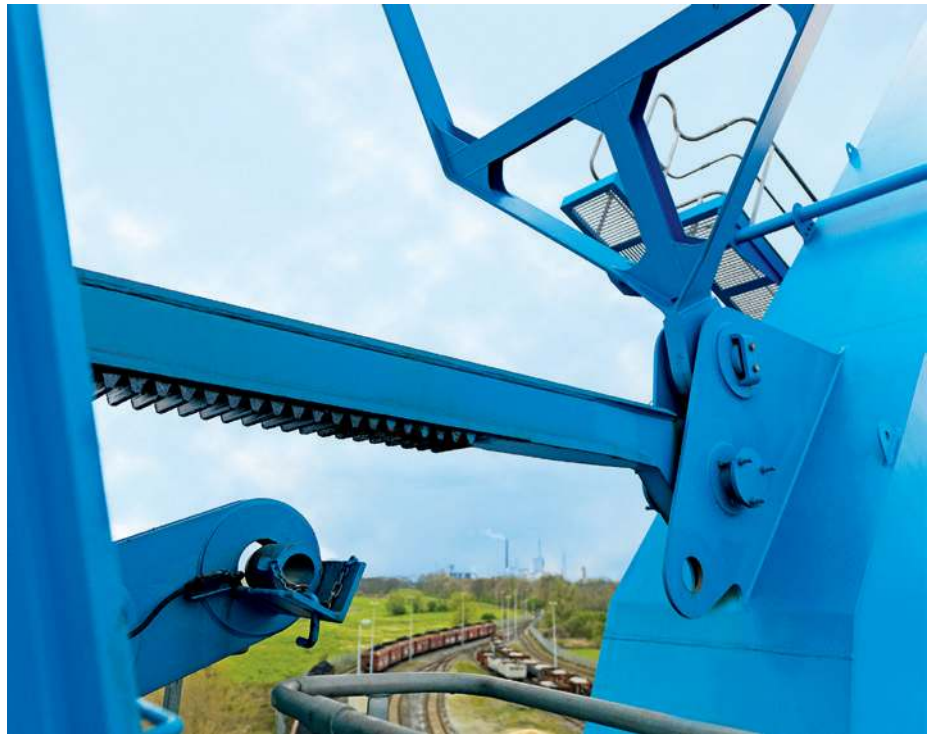
↑ Reliable and safe – rack and pinion derricking gears
