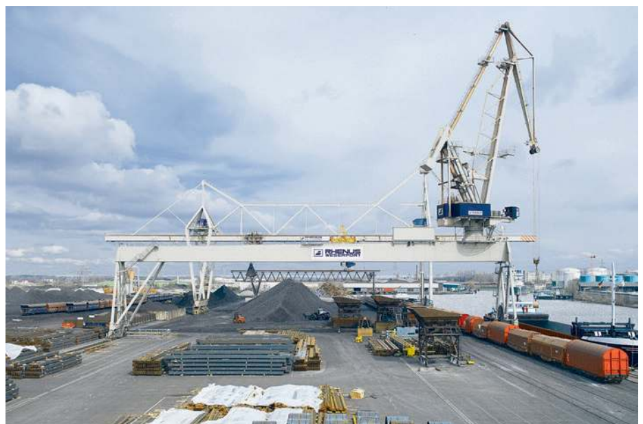
↑ Tukan with an asymmetrical gantry
