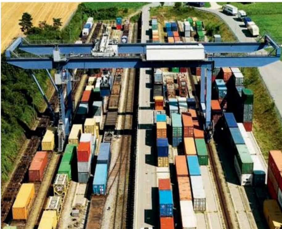
↑ The robust box girder design is perfectly suited to the Terminal Server's mode of operation
