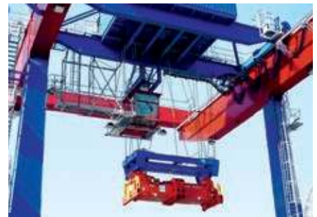
↑ Heavy duty trolley in double girder design (turnable head-block as option)
