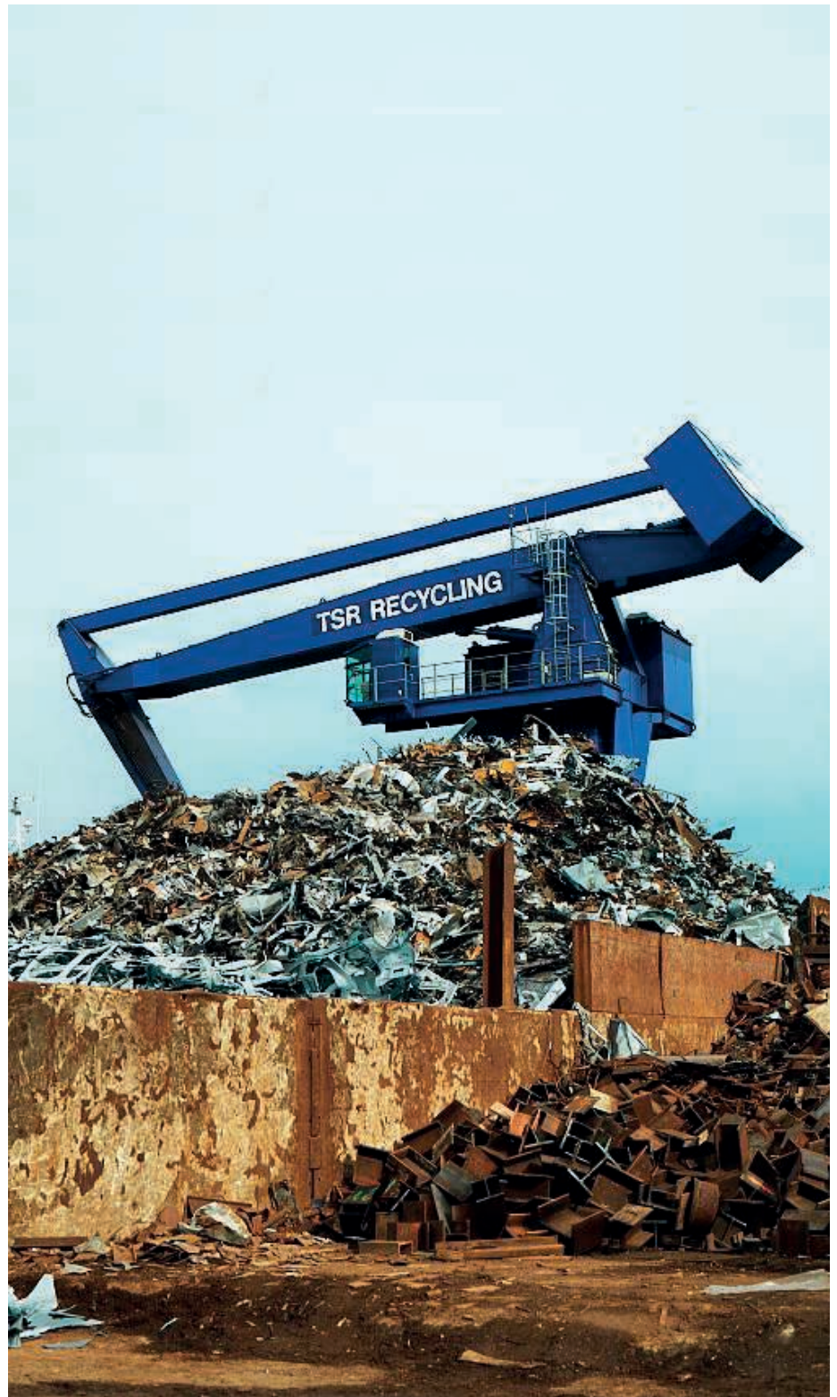
↑ The counterbalanced four-part boom system of the Pelikan
