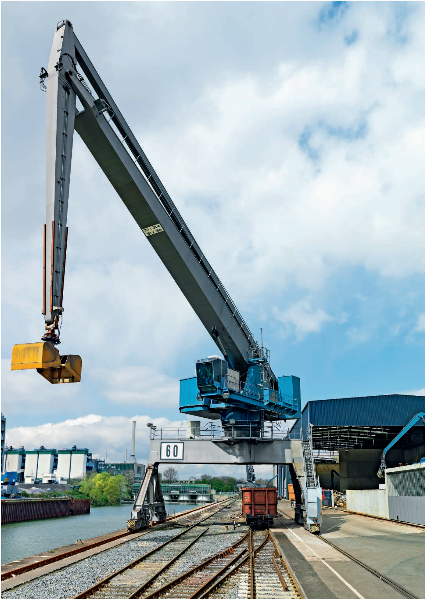
↑ The Pelikan with high portal on a rail undercarriage
