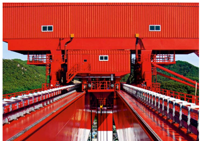
↑ Lower trolley with hooks between the girders, upper trolley with hooks on the right and left side outside the girders
