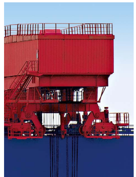
↑ Trolley Travel Mechanism of Upper Trolley
