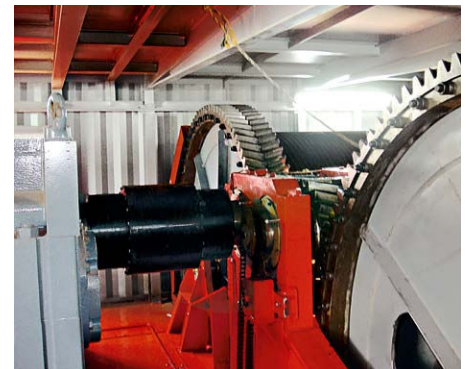
↑ Hoisting Mechanism of Lower Trolley
