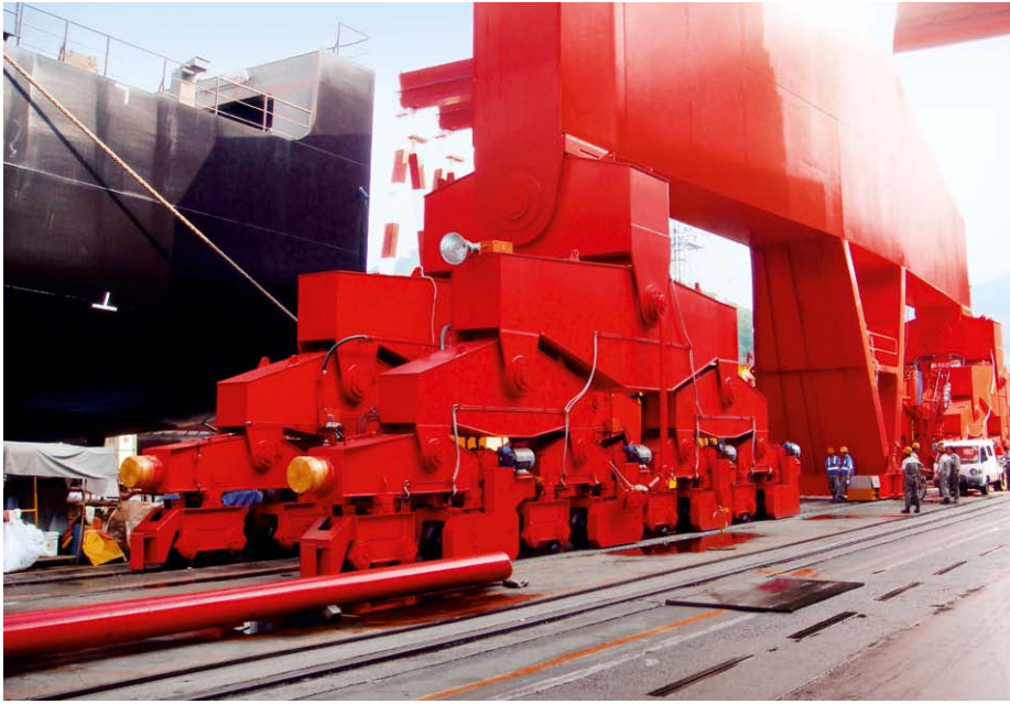
↑ Crane Travel Mechanism available in One Rail or Two Rail Design
