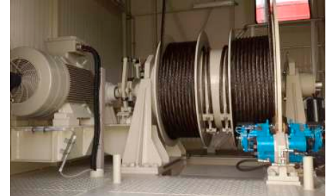
↑ Boom hoist gear
