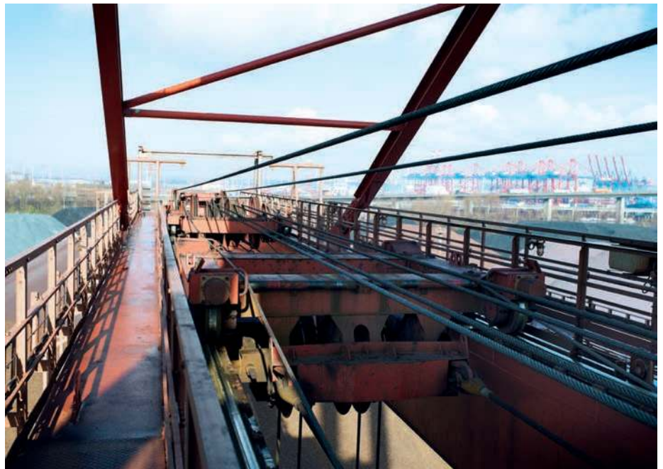
↑ Main and auxiliary trolley on twin girder boom
