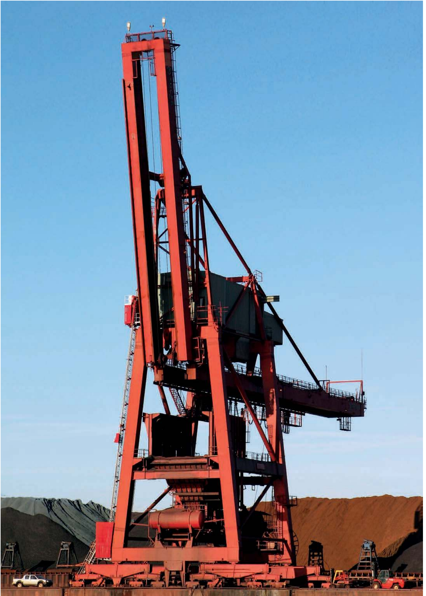
↑ Stability and rigidity of the gantry structure is the basis of high performance of the Digger
