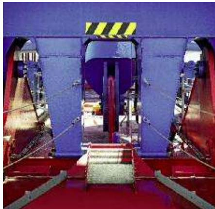
↑ Boom connection to gantry on waterside
