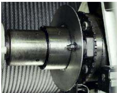
↑ Snag-load device integrated in the hoisting drive chain
