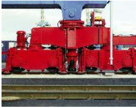
↑ Curvable travelling unit with guide rollers
