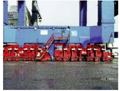
↑ Gantry drive unit
