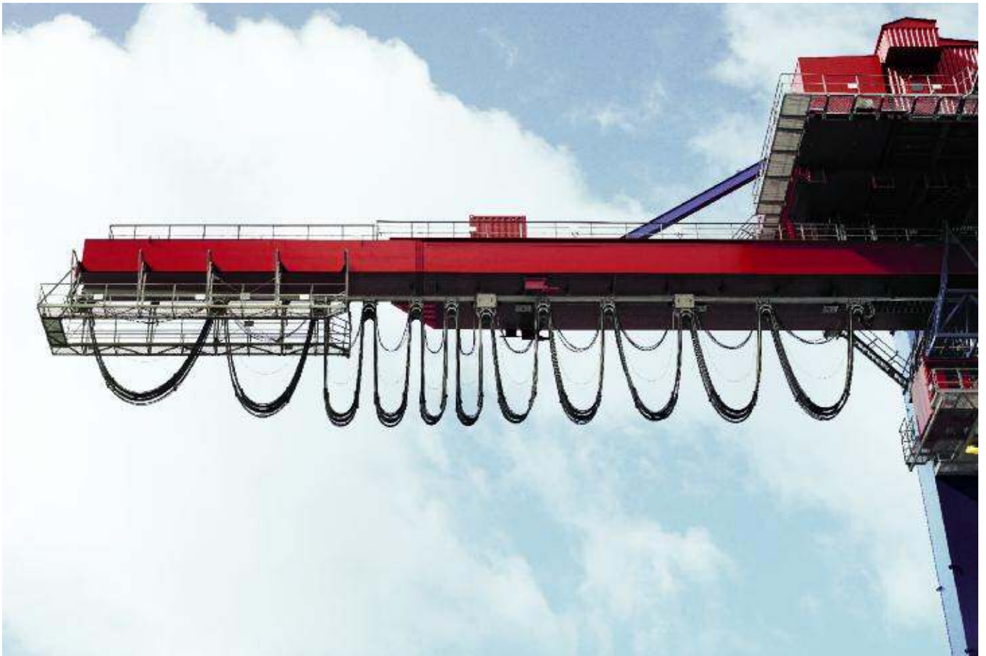
↗ Festoon system with driven carriages to harmonise acceleration
