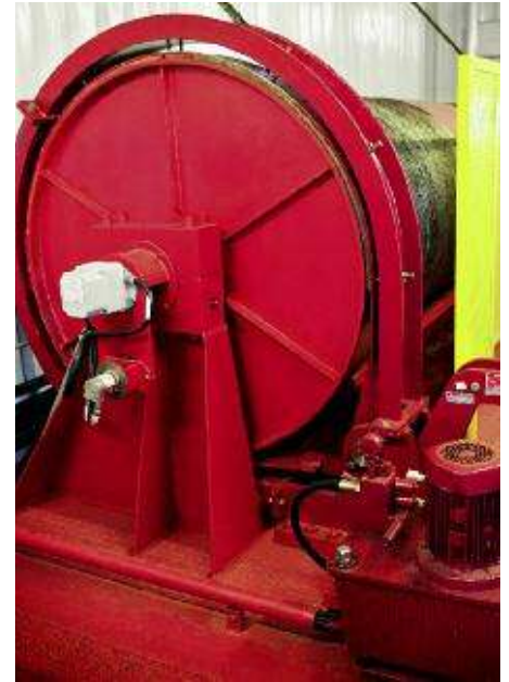
↑ Emergency band brake at boom hoist
