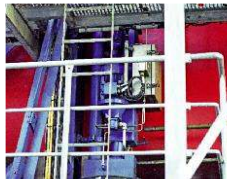
↑ Snag-load device acting on the rope fix point
