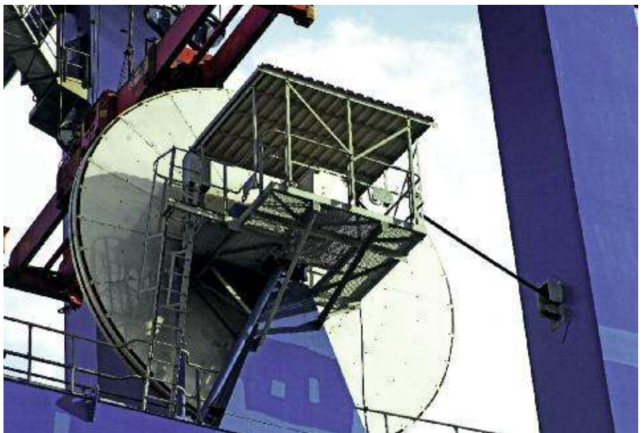
↑ Power supply by sealed spiral cable reel
