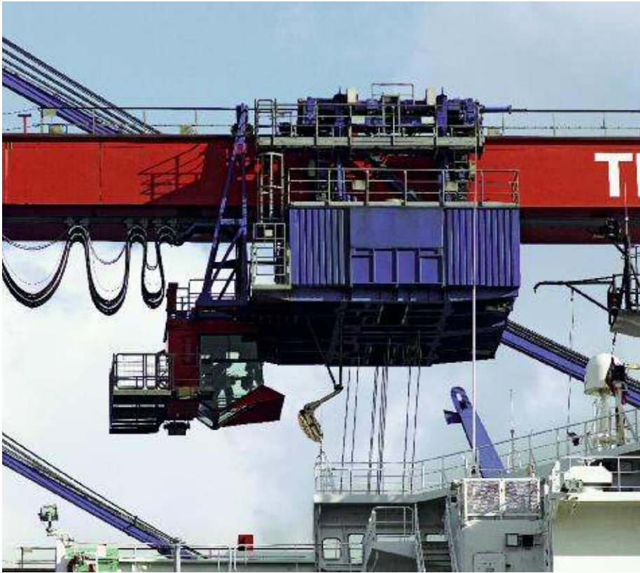
↑ Machinery trolley on mono box boom
