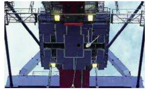
↑ Machinery trolley on the waterside boom
