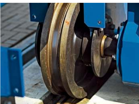
↑ Corner bearing for rapid wheel change
