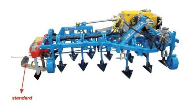
Cultivator with 30x30 spiral spring and cage rollers
