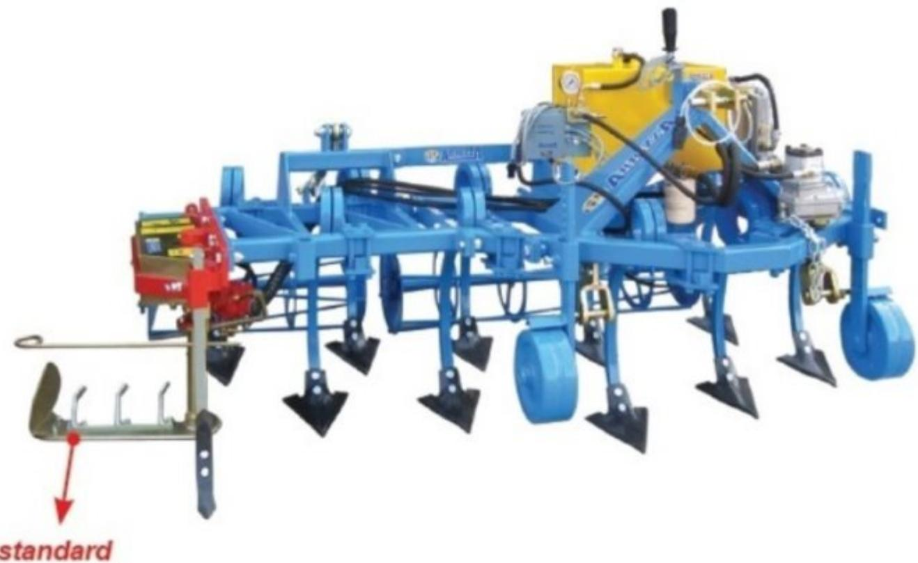
Cultivator with 30x30 spiral spring and cage rollers
