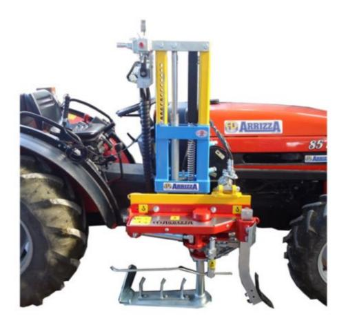
RH inter-row ventral kit with 45 - 55 - 65 cm inter-row blade plant lifting (to specify during the order) controlled by a single channel joystick for emergency return
