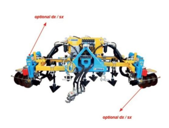
Cultivator with hydraulic widening, 30x30 loop springs with releasable rods and cage roller
