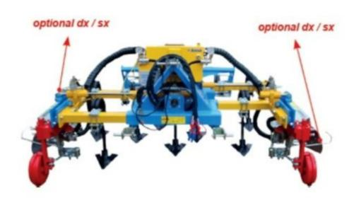
Cultivator with hydraulic widening, 30x30 loop springs with releasable rods and cage roller
