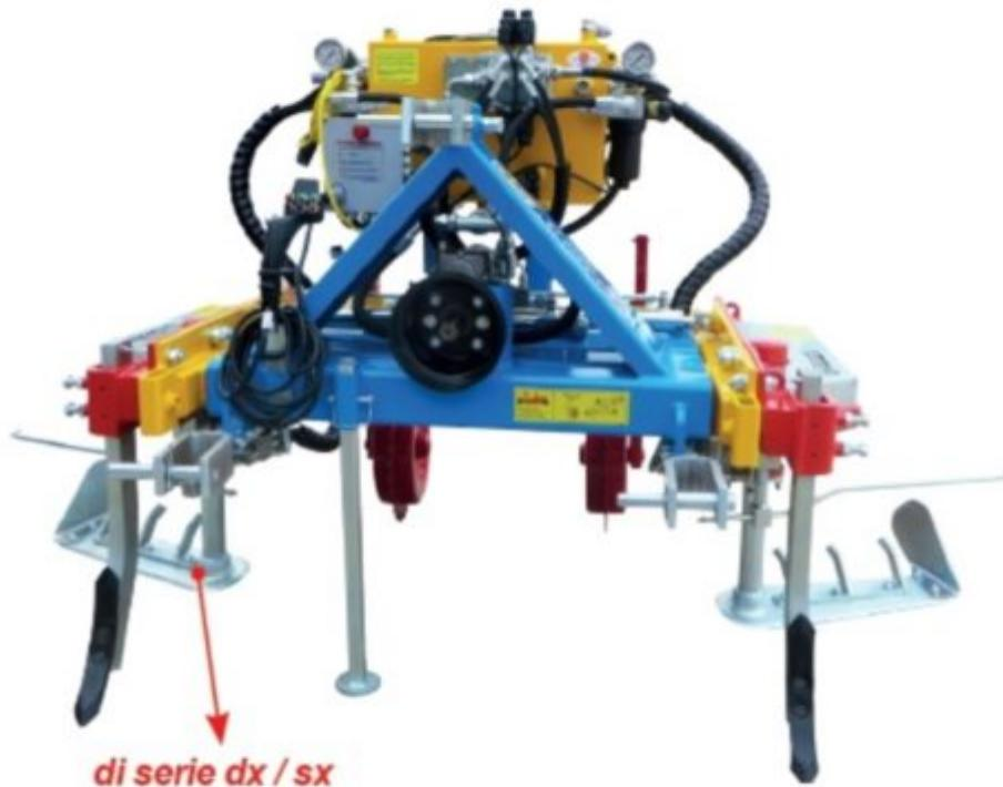
Tool-carrier with hydraulic widening
